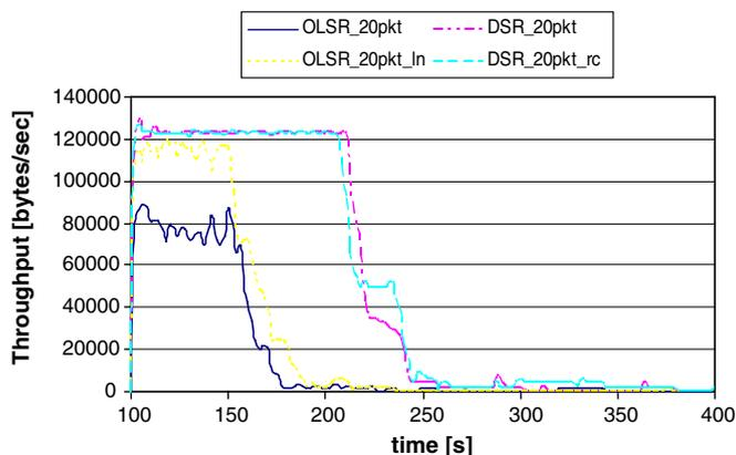
Fig. 10. Throughput vs time with fixed connection pattern.
