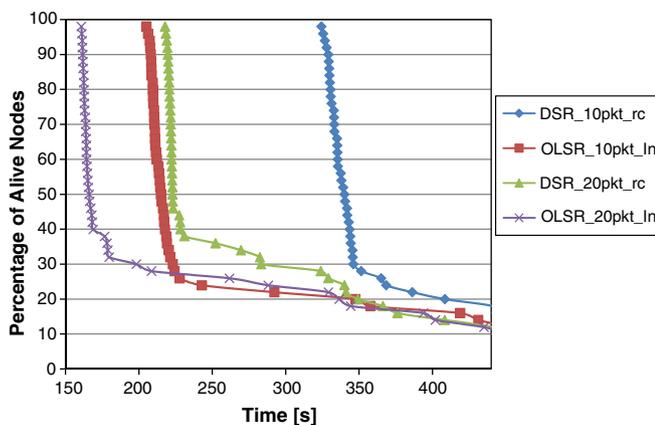
Fig. 8. Alive nodes vs time with fixed connection pattern and different data packets rate (10 and 20 pkts/s).
